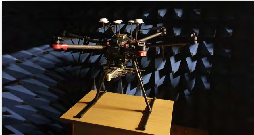
Specialized UAV Platform in our Full Anechoic Chamber.
