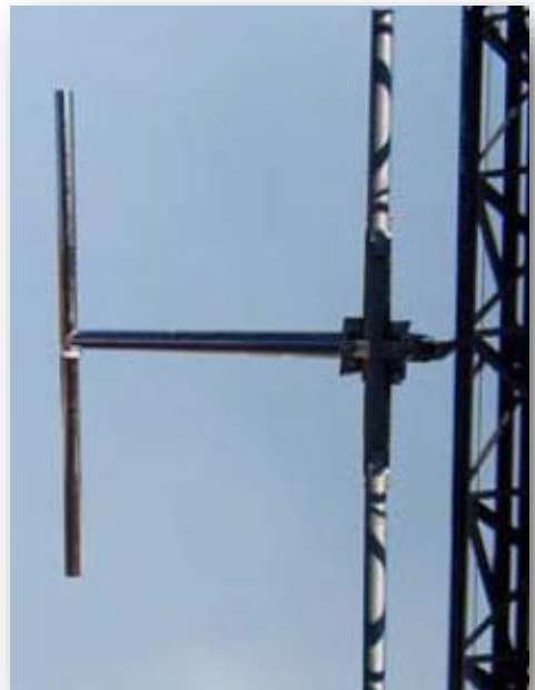
Example: A typical FM dipole antenna
